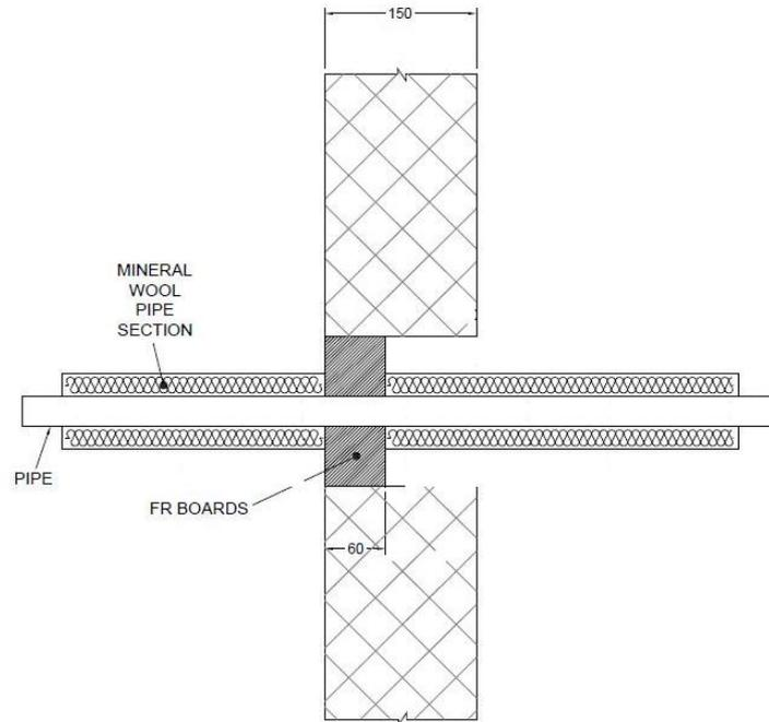
\* 600 mm long insulation required for Alupex pipes
