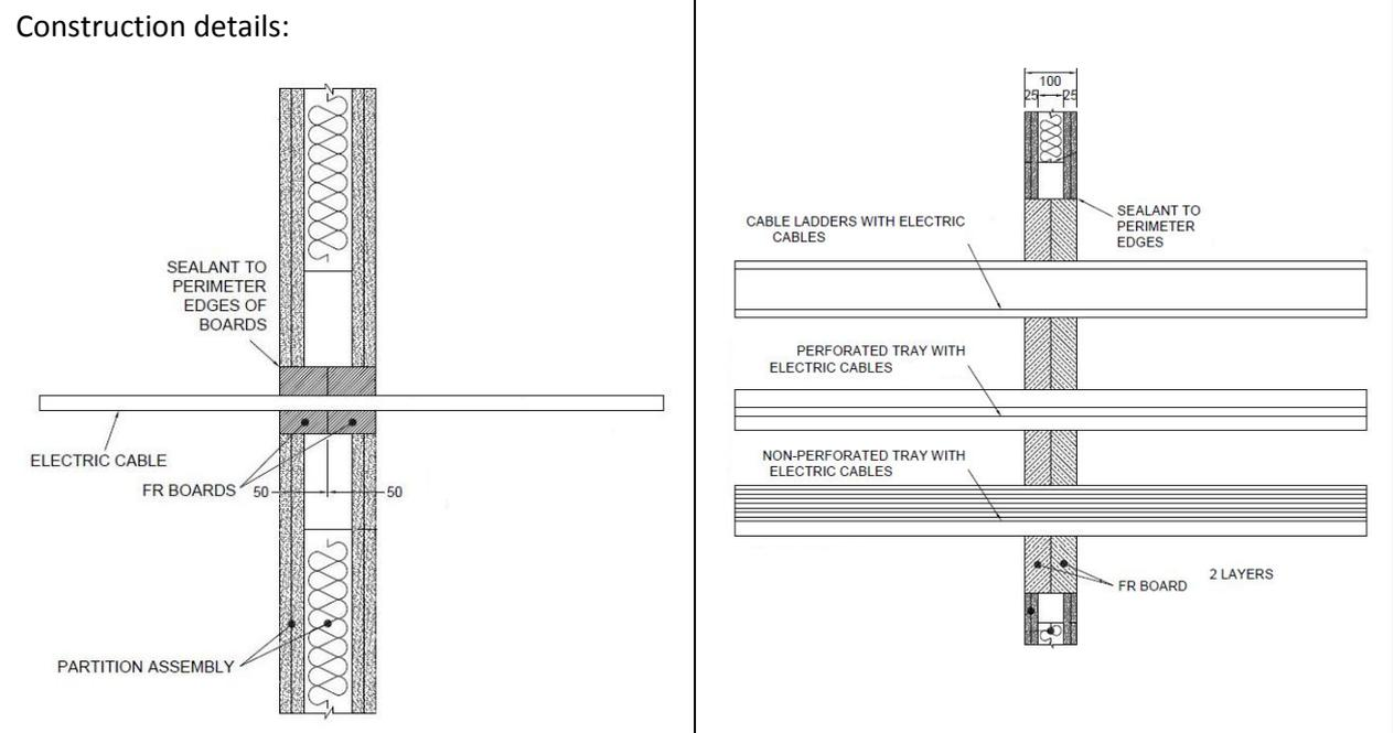
Note: Insulated metal pipes may also be included within the same seal as cables subject to minimum 100 mm separation. See separate classification for pipes.
